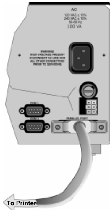
Figure 3-7 Parallel Printer Cable Connection to 9500
